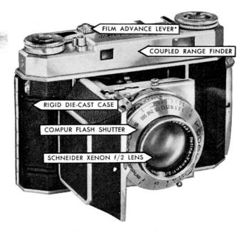
\*important: The film advance lever advances the film and cocks the shutter; it should not be forced. It locks when the counter is set at 1, also when the film has been advanced but not exposed.
